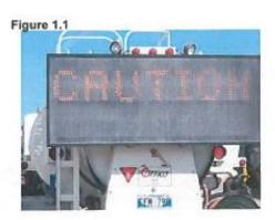
Figure 1.0 and 1.1: Tanker equipped with 4 beacons, retro-reflective striping and combined directional lighting/caution signage.
